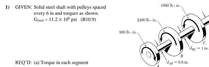
(b) Maximum shear stress in shaft. In which segment does it occur?
